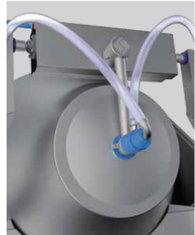
Automatic brine loading system
